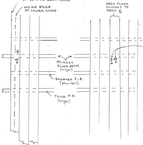
FOR GAUGES ATTACHED TO TOP OF DECK THERE IS SLIGHT CHANCE OF TRUCK BREAKING GAUGE, BUT IF DRIVER STICKS TO APPROX. CENTER OF BRIDGE TIRES SHOULD CLEAR GAUGES AT DECK Q.
