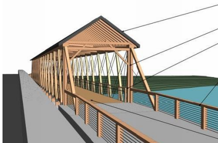
Diagram of reconstructed Bell Ford Covered Bridge Courtesy Hamilton County Parks and Recreation
